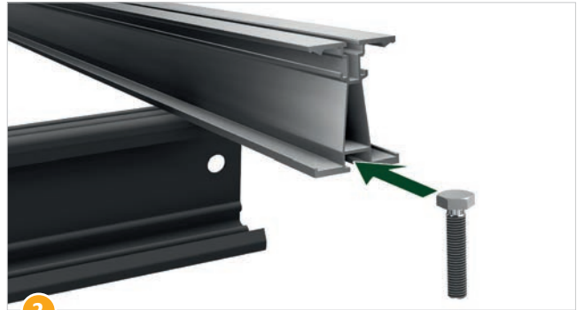
2 Insert the screw of the steel rafter clamp ( item no. 41502-00 ) into the lower channel of the rafter and push it up to the stop of the rafter-bearing girder.
