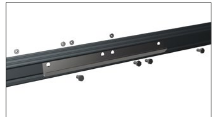
Connection of two steel purlins with hexagon screws
