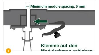
Push clamp over module frame. Attention: Do not damage back foil!
