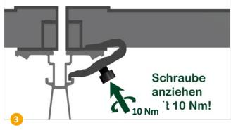
Tighten M6 bolt with a torque of 10 Nm.
