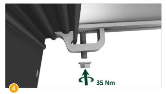
Fixate clamp by tightening the nut.
