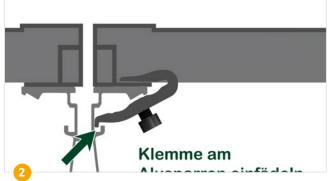
Insert clamp into aluminium rafter.
