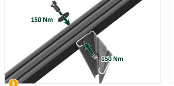
Fasten the rafter-bearing girder with a screw.
