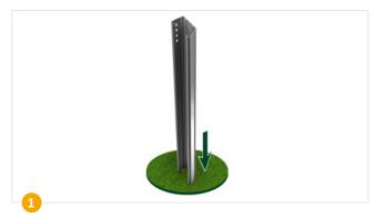
Install C-pile with a standard hydraulic pile driver in accordance with the respective ramming plan.
