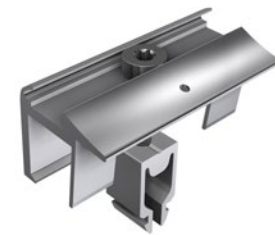
End clamp with grounding pin for frame heights 28 mm - 45 mm
