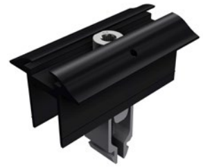
Mid clamp with grounding pin for frame heights 28 mm - 45 mm
