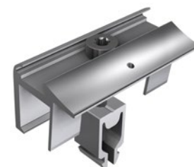
End clamp with grounding pin for frame heights 28 mm - 45 mm
