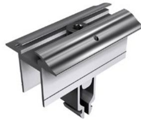
Mid clamp with grounding pin for frame heights 28 mm - 45 mm
