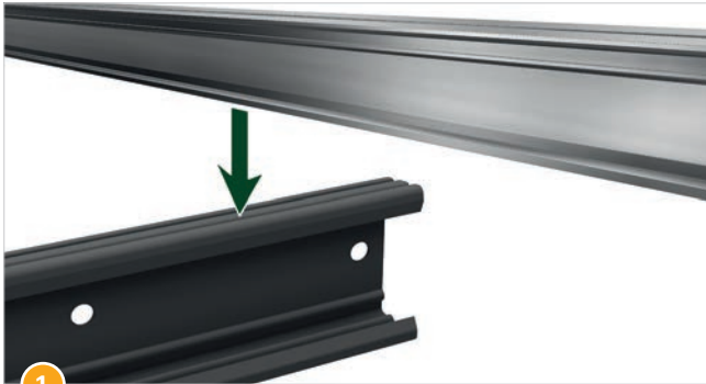
1 Position rafter on the rafter-bearing girder.
