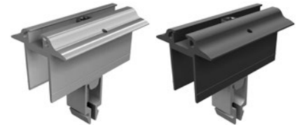
Mid clamp Vario without grounding pin for frame heights 28 mm - 50 mm
