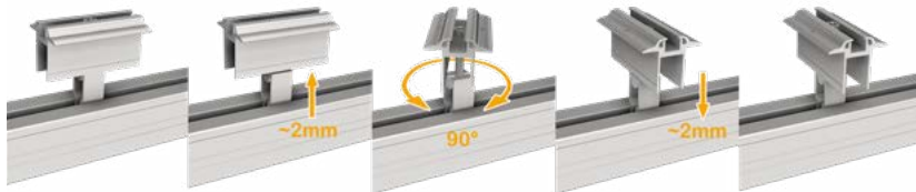
Horizontal or vertical by simply lifting and rotating the clamp
