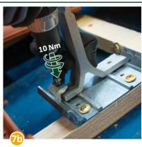
Fixate it by tightening the bolt to (10 Nm).
