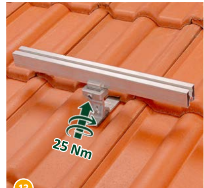
13 Fixate the Clamp Combination by tightening the bolt (25 Nm) – done!
