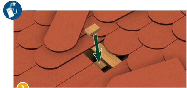
2 Place a shim or wooden wedge on the sub-structure to compensate for the height difference.
