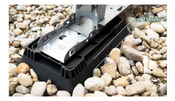
1. Lay out the Fast Flat Basic Frames as usual. Gently embed the SL Rack Base Plate Gravel (item no. 22300-85) into the correct position in the gravel or substrate.
